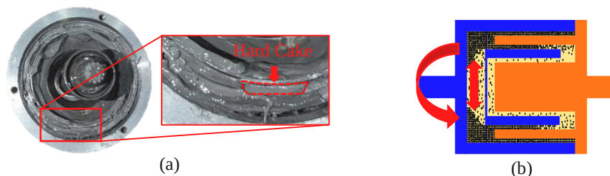
Figure 1: (a) Resulting hard cake between the clutch drums (b) Clutch cross-section schematic of centrifugation
